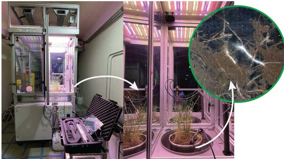
Fig. 1. Tall wheatgrass monoliths were excavated and relocated to the Berkeley Lab for incubation in the EcoPOD. The image shows the EcoPOD housing the plants with connected minirhizotrons. The upper inset image shows an image of roots photographed with the minirhizotron camera.
