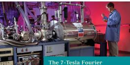
The 7-Tesla Fourier transform ion cyclotron resonance mass spectrometer at the William R. Wiley Environmental Molecular Sciences Laboratory. Mass spectrometry is the most sensitive method for identifying proteins.
