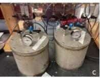
*Figure 6 Pressure vessels for incubation of plates anaerobically*
