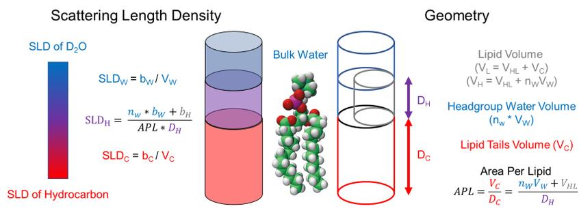
Figure 2. Implementation of the slab model for symmetric lamellar structures, shown here on a per lipid basis in one leaflet. Our implementation in Tan et al. (2021) provides a self-consistent fitting algorithm to extract the key parameters of area per lipid (APL) and water content in the head group region ( $n_H$ ).
