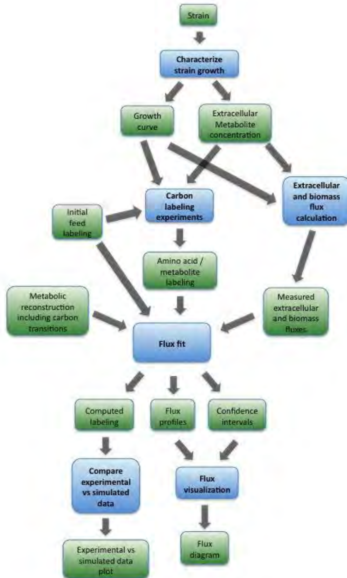
Figure 1. Workflow for ^{13}\text{C} metabolic flux analysis. Blue blocks indicate processes (e.g., experiments or algorithms), and the green blocks indicate datasets or physical objects. See text on next page for callout to this figure.
