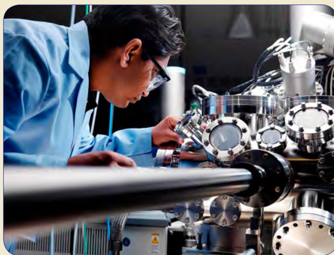
Fig. 9. Time-of-Flight Secondary Ion Mass Spectrometer. [Image courtesy DOE EMSL]
