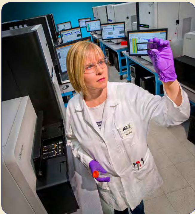
Fig. 8. Illumina HiSeq Sequencing Units and Flow Cells. [Image courtesy DOE JGI]
