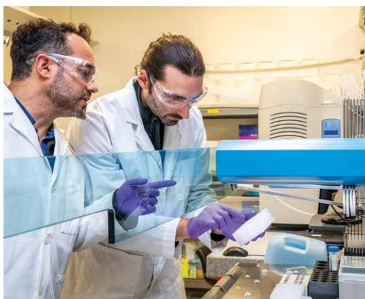
BioLector Microbioreactor. JBEI scientists work with the BioLector instrument to understand the microbial production of biofuels and bioproducts. [LBNL]
