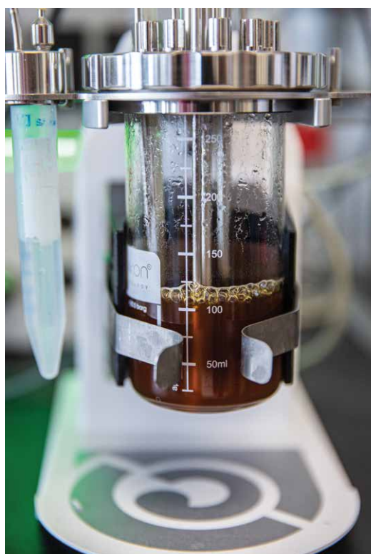
Hydrolysate Fermenters. A hydrolysate experiment in process in GLBRC’s Experimental Fermentation Facility. [GLBRC]
