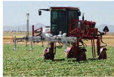
High-throughput phenotyping tractor deployed in Maricopa, Arizona. Bottom image shows georeferenced crop canopy temperatures overlaid on the field map. (Courtesy Matt Conley, USDA Agricultural Research Service)
