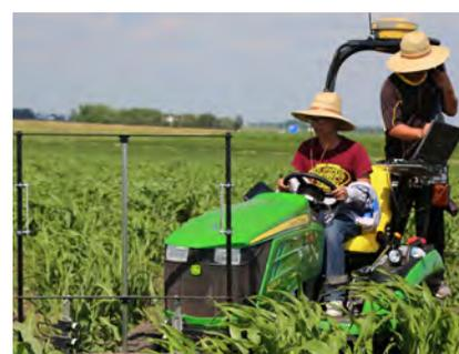
New field-based technology will digitize and screen for biomass yield traits. The converted John Deere tractor "robot" has a GPS-enabled auto-steer function and sensors. Researchers "train" its function to follow a specific route. (Courtesy Patrick Schnable, Iowa State University, Ames)
