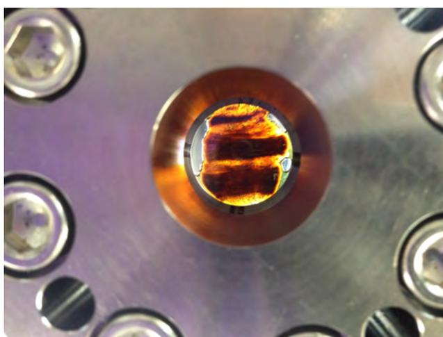
*New improved temperature-pressure cell to perform in situ SANS experiments of thermochemical pretreatment of biomass.*
