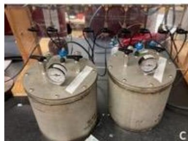
**Figure 6** Pressure vessels for incubation of plates anaerobically
